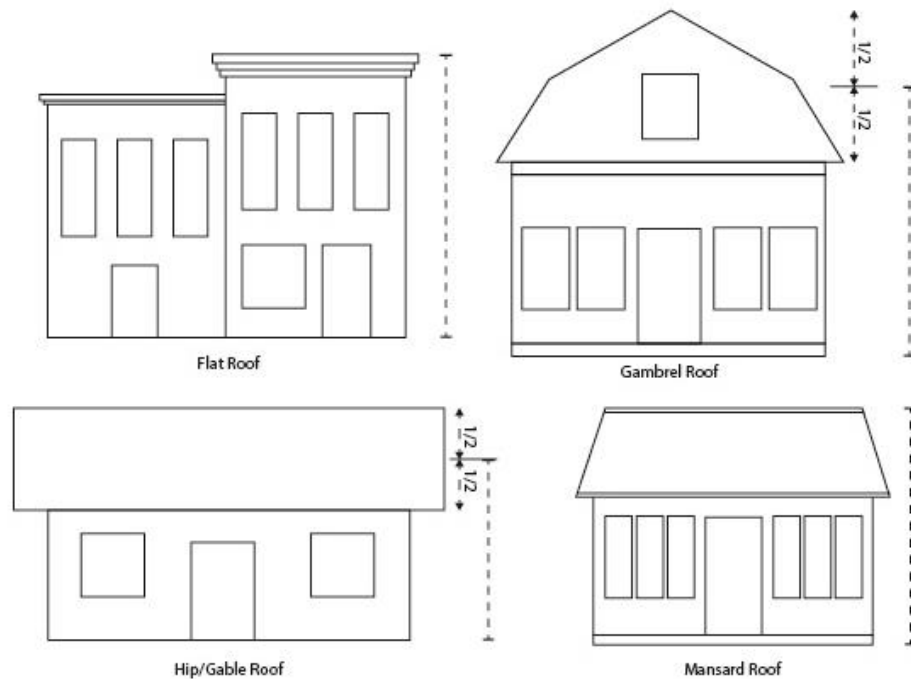
Figure 5.3 | Building Height Measurements
